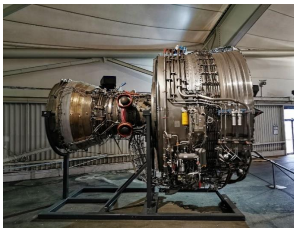
Slika 2. Rolls-Royce Trent 900 i Engine Alliance (GE i Pratt & Whitney) GP 7200 [2, 3].
